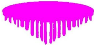
Air pressure too low or fluid flow too high
