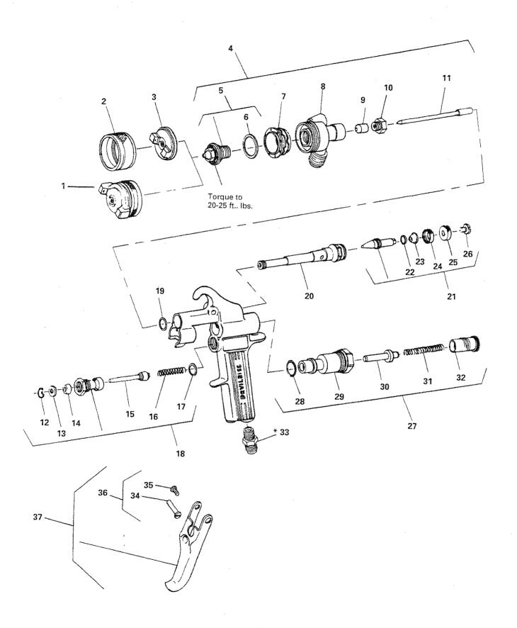
\*Apply thread sealant (i.e. Loctite 242, blue or equal) on threads.
