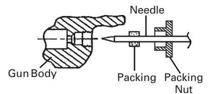
1. Remove adjusting knob and needle spring from gun.
