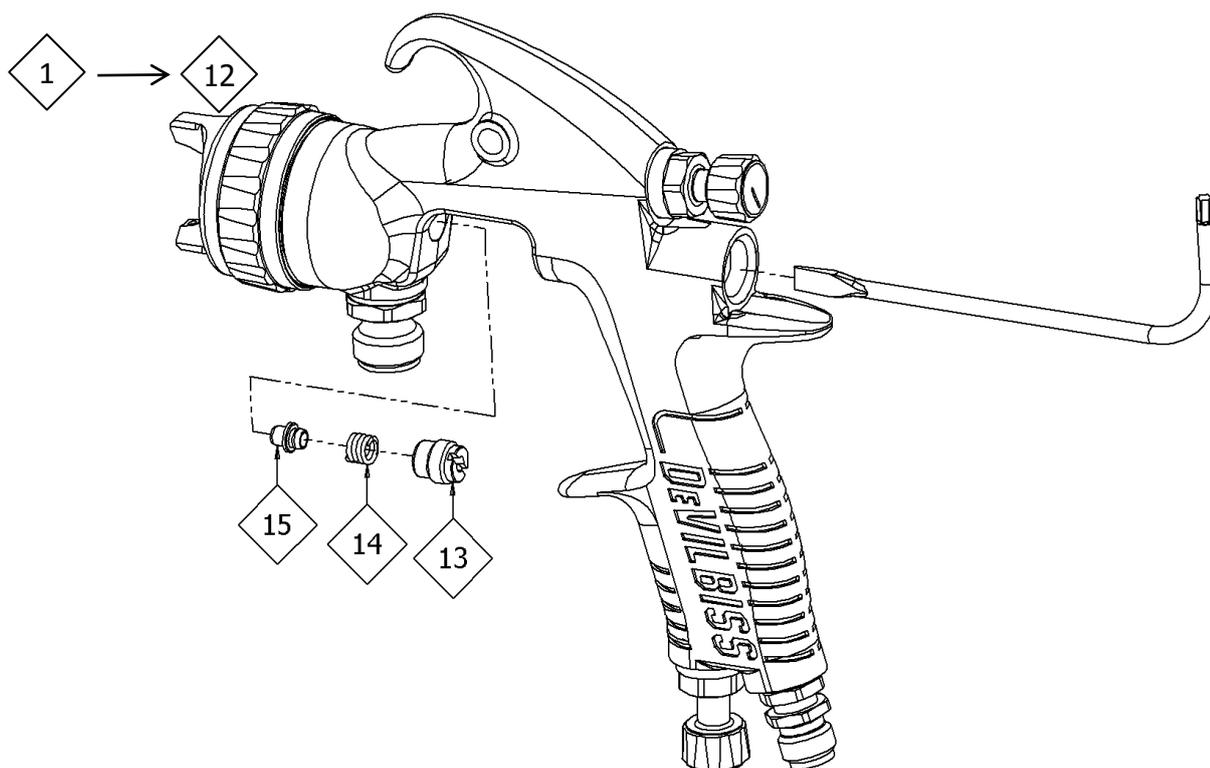
**REPLACEMENT DE LA VALVE DE RÉGLAGE DU JET**
