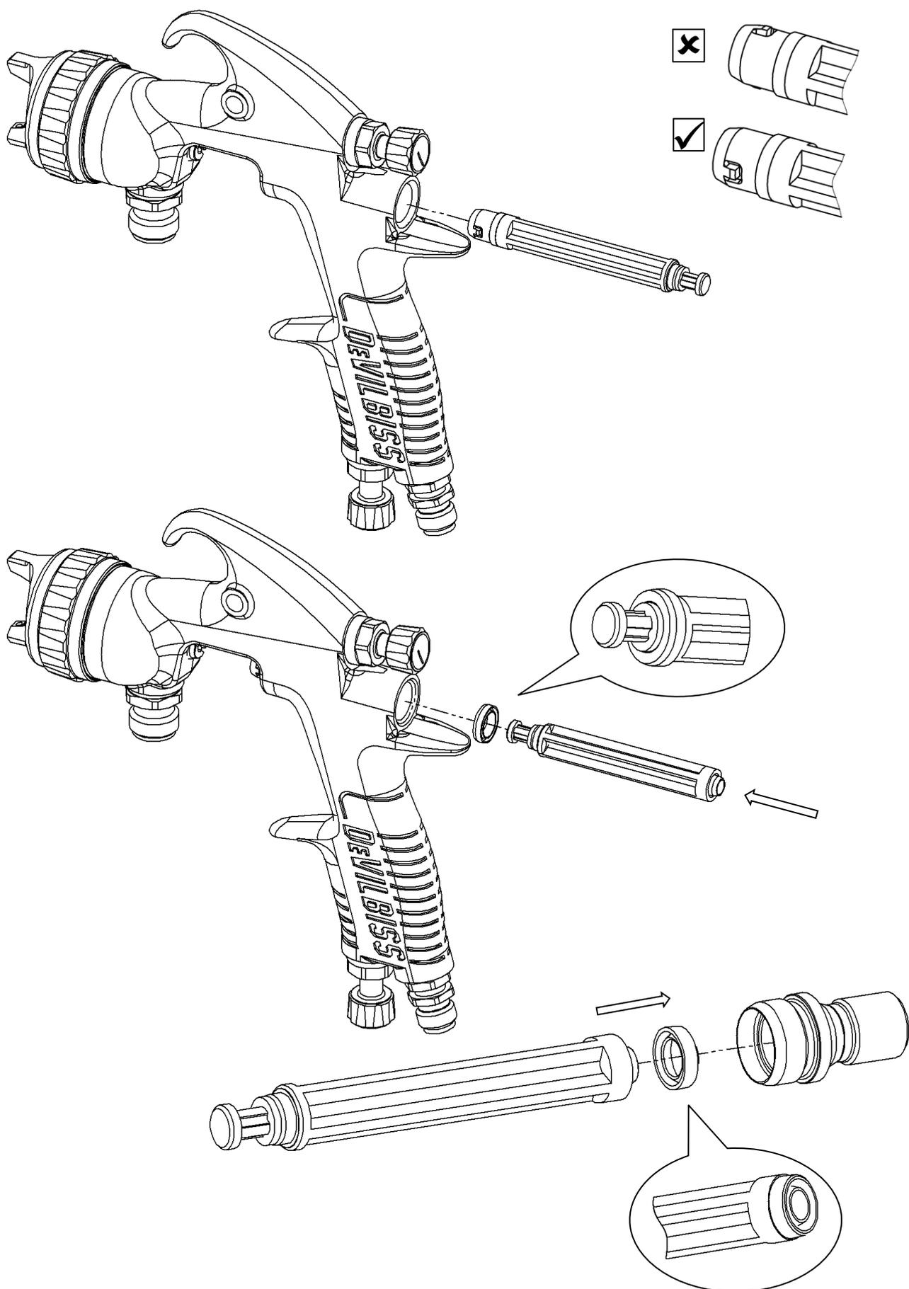
**DÉSASSEMBLAGE DU PRESSE-ÉTOUPE****PAGE 13 - DÉSASSEMBLAGE DE LA SOUPAPE D'AIR**
