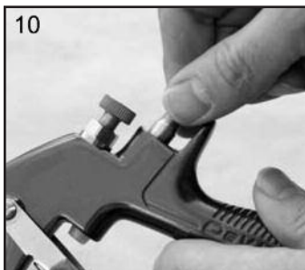
10. Fit new Front Air Valve Seal to gunbody and press firmly to ensure Seal is engaged.
