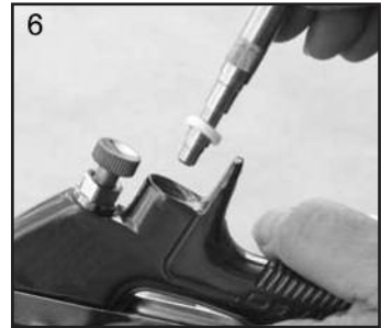
6. Retirer le support de la soupape.
