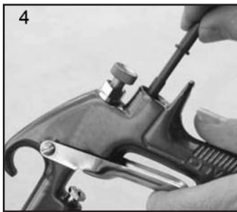
4. Remove Air Valve Spindle (11).
