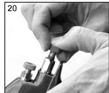
20. Fit Fluid Needle Spring (8) and Needle Adjusting Screw (7).
