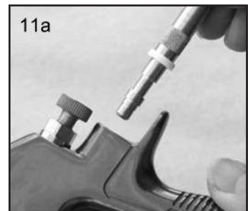
9. Fit New Front Air Valve Seal to Service Tool so that the groove faces the handle end of tool.
