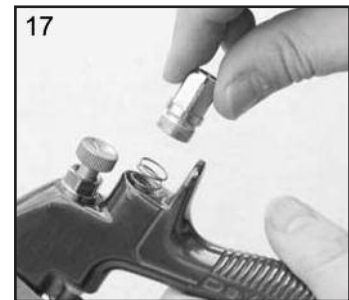
17. Replace Airvalve Spring by inserting small end of spring into gun, and screw in Housing (10).
