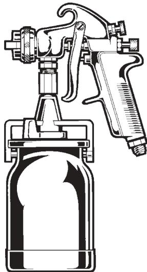
**Figure 1 Suction Feed Gun with Attached Cup**
